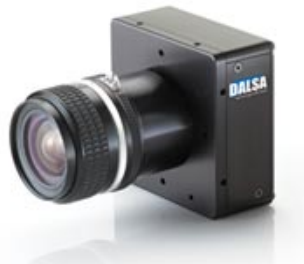
2352 x 1728, Medium Camera Link, 62 fps, 7.4 um, 10 bit Camera
