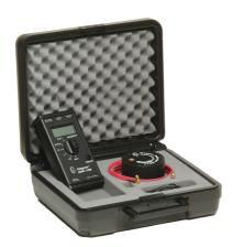
The Hagner ERP-105 Digital Photometer is a precision instrument designed to measure the luminace of photoluminescent signs and materials over a range of  $0.01 - 20,000 \text{ mcd/m}^2$  ( $0.00001 - 20 \text{ cd/m}^2$ ), in the field as well as in the laboratory.
