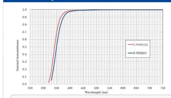
Internal transmittance of S-PHM52Q has been improved comparing with S-PHM52
