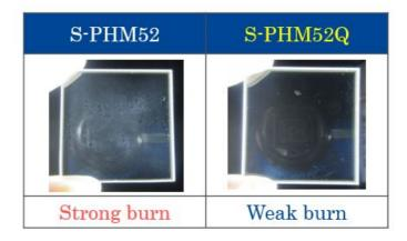
Provided this test to check the burn on the polished surface
