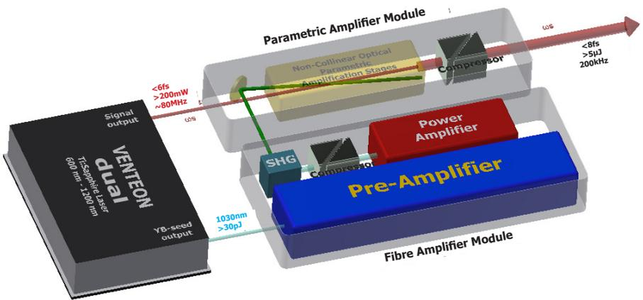
The **venteon dual** as an ideal front-end for OPCPA seeding since it offers two separate outputs. The ultrabroadband signal with a pulse duration of  $<6\text{fs}$  and a seed output at  $1030\text{nm}$  and  $>30\text{pJ}$  for subsequent power amplification. No nonlinear broadening of the Ti:sapphire spectrum is needed, resulting in excellent stability and intrinsically low jitter between the two outputs.
