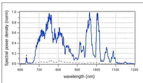
Fig. 1. Amplified output spectrum of the **venteon OPCPA** (blue) and initial signal seed spectrum of the broadband **venteon dual** seed oscillator (black). Due to the ultra-broadband gain characteristic of the parametric process, nearly the whole seeded bandwidth becomes amplified enabling pulse durations <8fs.
