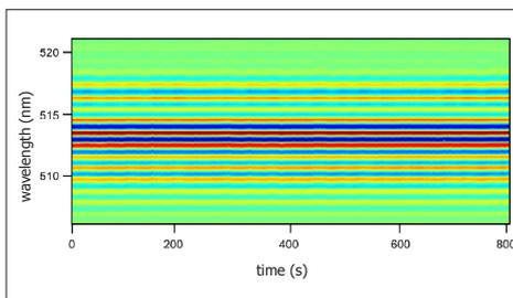
Fig. 4. Output CEP stability of the **venteon OPCPA** measured with an second f-to-2f interferometer for the compressed output. A slow feedback loop to the seed oscillator is used for the stabilisation. The system features an rms phase error smaller than 100 mrad (measured over more than 10 min @ 3ms integration time).
