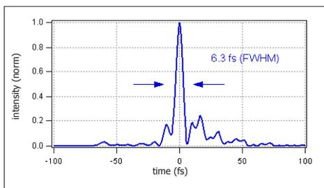
Fig. 2. Compressed output pulse of the **venteon OPCPA** system measured with **venteon SPIDER**. The few-cycle pulse duration together with the ability for a CEP stabilisation (see below) and pulse energies with  $\mu\text{J}$ -levels, make this system ideally suited for e.g. attosecond science and nonlinear spectroscopy.
