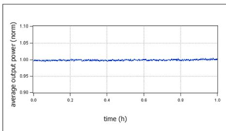
Fig. 3. rms noise of the **venteon OPCPA** output after system warm-up time. This exceptional low-noise output performance can be achieved even without an active power stabilisation e.g. controlling the delay stages within the NOPA process.
