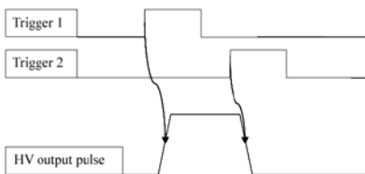
Fig. 3. Control timing charts for two-pulses controlled drivers
