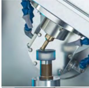
Deterministic aspheric polishing.
