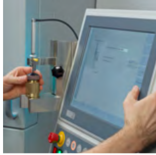
Center thickness is directly measured at the machine.
