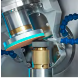
Economical, flexible and fast polishing of aspheres.
